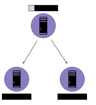
When a client makes a request, the server requests a slot in the log to apply a command, the "prepare" phase.
