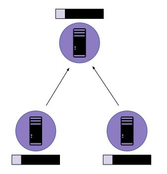
If a majority of servers responds to the prepare phase, the originating server, will send the command to be applied to the log in that spot, the accept phase.
