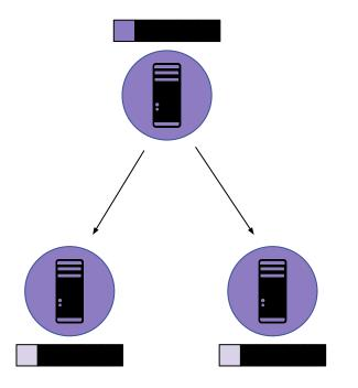
If a majority of servers responds to the prepare phase, the originating server, will send the command to be applied to the log in that spot, the accept phase.
